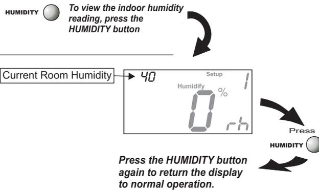
NOTE: Due to variations in environmental conditions, it is not always possible to achieve the desired humidification or dehumidification setpoint.
