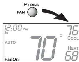
**Fan On** indicates constant fan operation. If Fan On is selected the fan will run continuously at all times, except in Off, **and** will only run if there is a heating or cooling demand in Unoccupied periods. Pressing the FAN button toggles this feature on or off.
