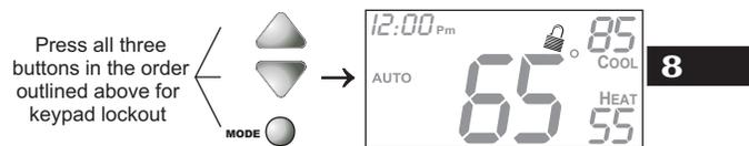
To **unlock** the keypad, press and hold the MODE button. While holding the MODE button, press the UP and DOWN buttons together. The
