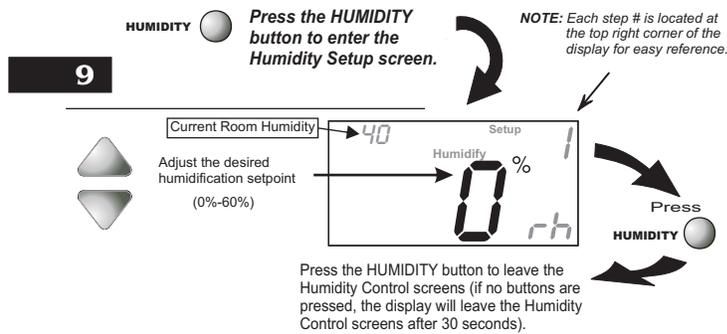
**Humidification Notes:** Press the
