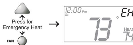
**OPERATION:** During Emergency Heat operation the thermostat will turn on the fan and the 2nd stage of heat when there is a demand for heat. Also during Emergency Heat the 1st stage of heating or cooling will be unavailable.
