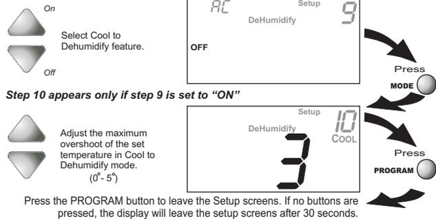
**Dehumidification Notes:** The thermostat must be in the Cool, Auto, or Program On mode for the Cool to Dehumidify feature to be available.
