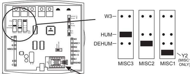
\*The Humidity Module (sold separately) must be installed to operate a humidification and/or dehumidification system.
