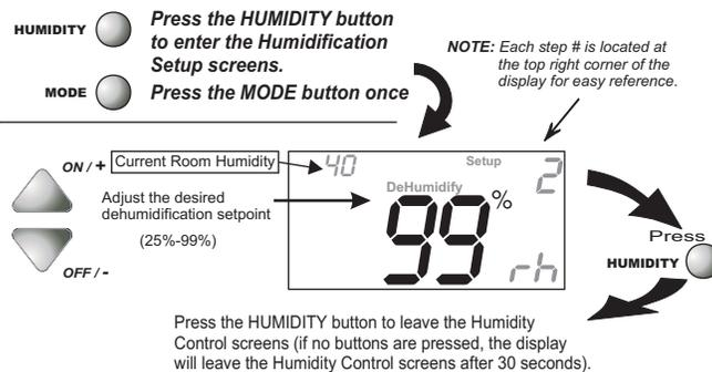
**Dehumidification Notes:** Press the button to set the dehumidification setpoint to 99% for no dehumidification operation. This will lockout Advanced Setup steps 9 and 10 (see page 10.4).
